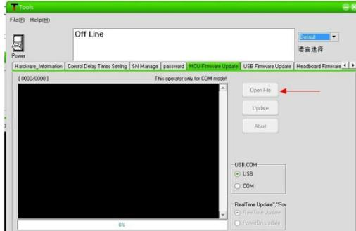
7: In the dialog box, locate the latest mainboard MCU firmware: select MB5.1.1.bin, click Open.
