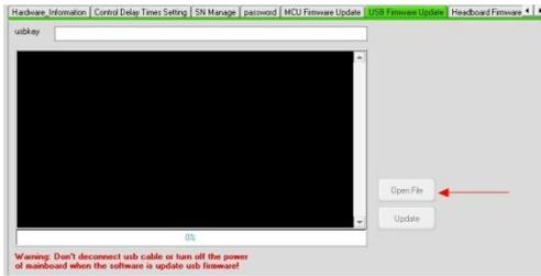
13: In the dialog box, locate the latest USB firmware: select USB5.1.6.iic, click Open.
