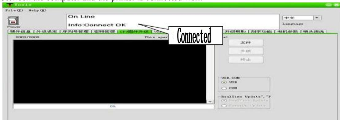
5.Turn on the power and open the mainboard.exe, then click the "Power", if the info shows connect ok, that means that the computer connect with the mainboard successfully.
